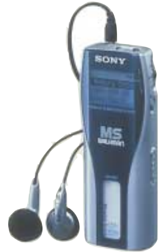
This Memory Stick Walkman, which went on sale in December 1999, employs a MagicGate Memory Stick to offer a new way to enjoy music. This IC recording media incorporates technology to prevent unauthorized copying, making the Walkman the industry's first product to conform to SDMI (Secure Digital Music Initiative) standards for the protection of digital music content.
