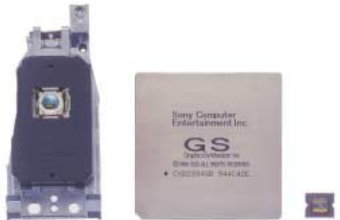
The PlayStation 2 game console employs nine devices produced internally within the Sony Group. Shown above are, from right, a dual-wavelength semiconductor laser coupler with DVD/CD compatibility, the Graphics Synthesizer image rendering engine, and an optical pickup.
