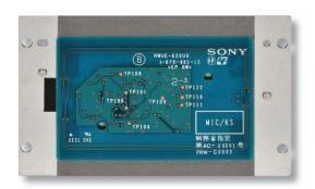
The RC-S620/S is a compact NFC reader module. Available with UART interface and suitable for incorporating into various devices, such as consumer devices, embedded system devices, and so on.
