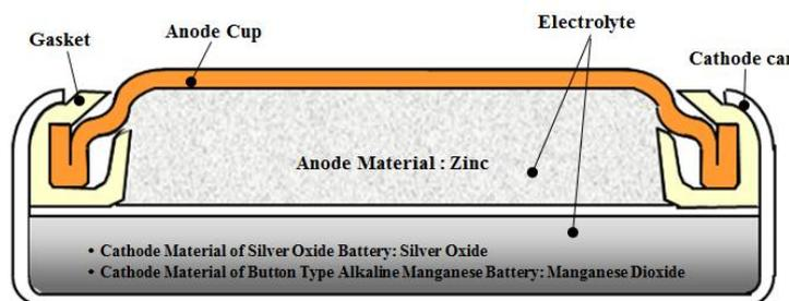
Fig.1: Cross section of button batteries
