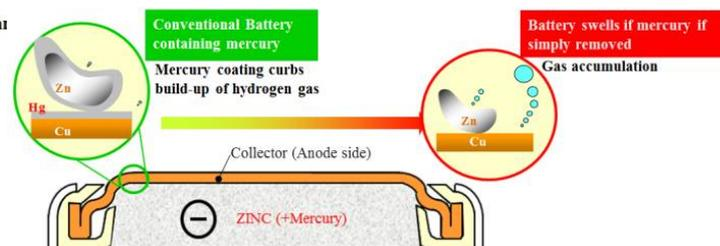
Fig.2: Role of mercury in conventional button batteries
