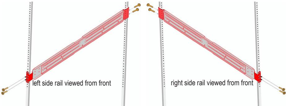
*Place enclosure into the mounting rails*
