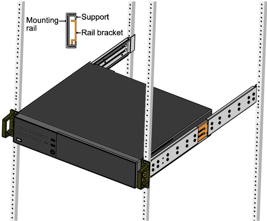
3. Insert the rail brackets attached to the enclosure into the rails.
