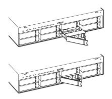
Reinsert the HDD lock removed in step 1.
