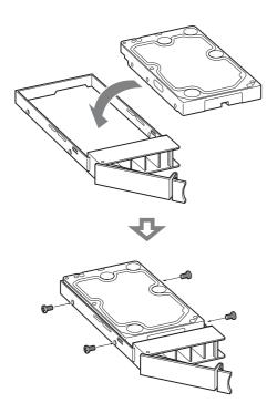
Fully insert the tray in which the HDD is installed into the slot, and lock it into place.
