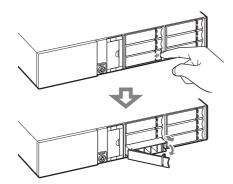
Remove the dummy HDD from the tray, set the actual HDD into the tray in the direction illustrated, and secure it using the four HDD screws (+K, UNC × 5).
