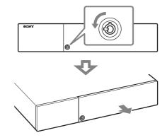
**2** Remove the HDD lock for the slot in which the HDD will be installed.
