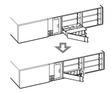
Reinsert the HDD lock removed in step 2.
