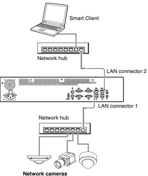
Connect LAN connector 1 to the same network as the network cameras.
