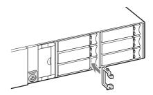
**7** Reattach the front cover, and lock it using the HDD cover key.
