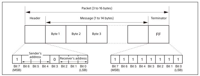
Fig. 2 Packet structure
