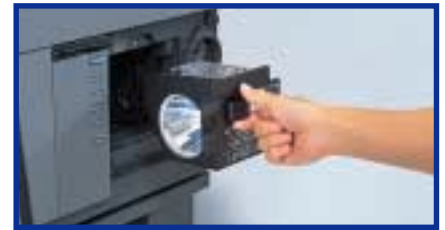
Replaceable high-brightness lamp
