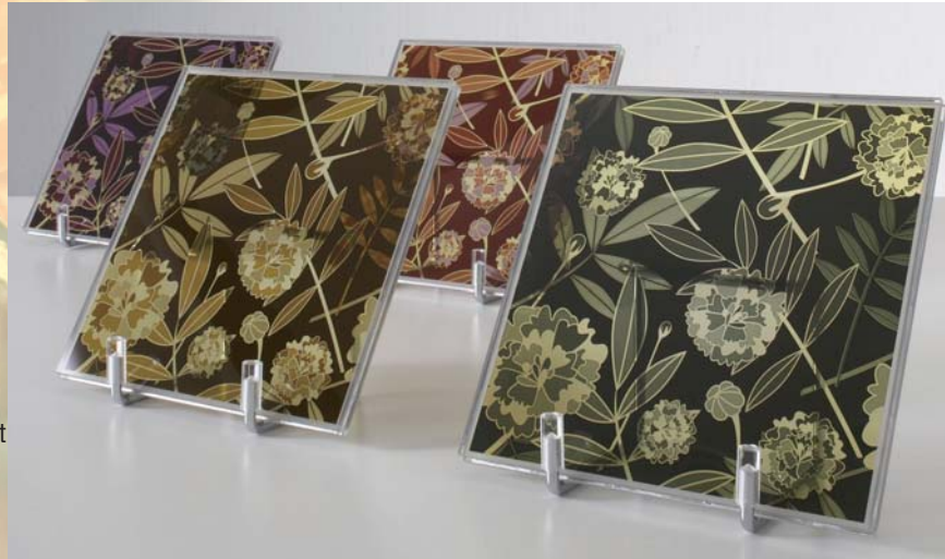
Prototype dye-sensitized solar cell panel. Screen printing is used for each of the four dyes, and a picture of marigolds is formed by applying colors with four levels of density.
