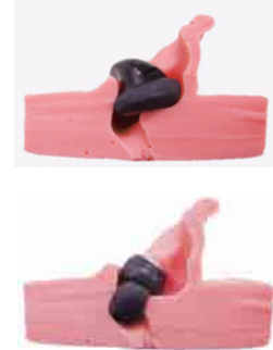
Cross section of ear casts showing the inserted state of in-ear headphones (the lower figure shows a closed type in-ear headphone)
