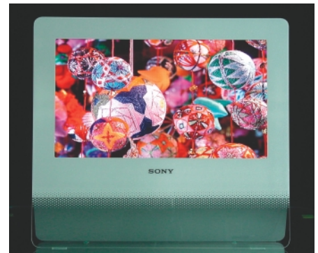
■ Photograph 2 Sony Color Filter Color Selection White EL Panel (12.5 type) Displayed at SID 2004
