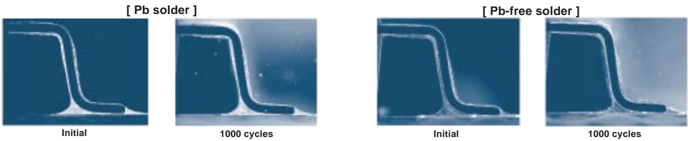
■ Photograph 1 Cross-Section Observations of Sn-Bi Plating Mounting
