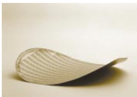
■ Photograph 1 Wafer with a 50 \mu\text{m} Thickness
