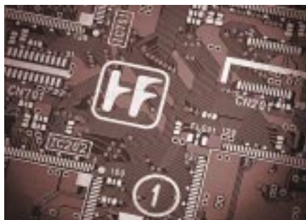
Photograph 1 Halogen-free Multilayer DVD Circuit Board (4 layers) and the Sony Halogen-free Mark, Which Is a Registered Trademark
