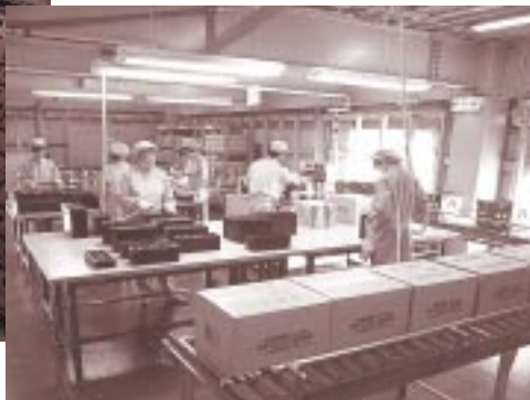
Inspection and final cleaning operation using tray automation
