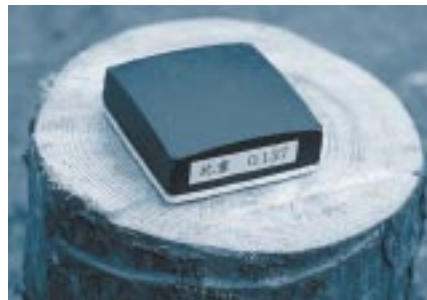
An ultralight weight, extremely heat-tolerant tile whose surface has been glazed. Current specific gravity is 0.132.
