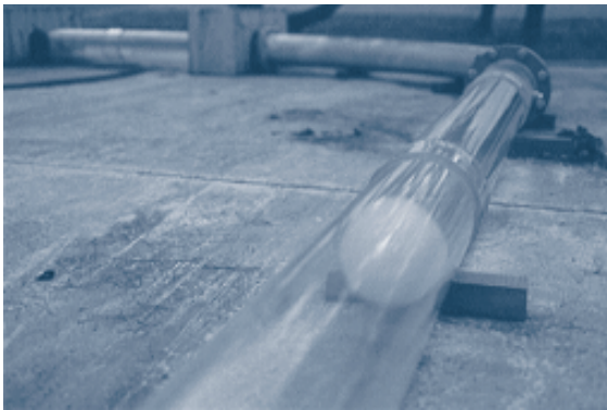
Snowballs travel through this 15 cm-diameter pipe at 8 meters/sec. (28.8 km/hr), a very impressive speed when viewed at close range.
