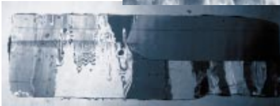
Vertical cross-section of an ice sample from the M-Wave rink. On the right, icicle shoots have been inserted to take advantage of their slicker end-face surface. On the left is a conventional rink. The rink employing icicle shoots has about 20% less friction.
