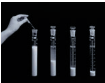
■ Coagulation using coagulants made from discarded plastic
